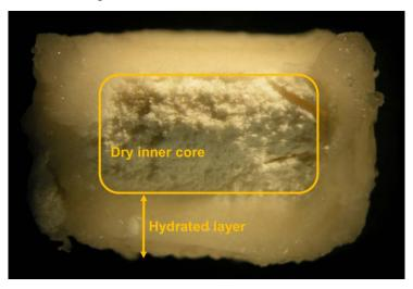
**Fig. 2.** Macroscopic view of PFS04 floating tablets (sodium alginate: 35.15 %; L-HPC 11: 25.0 %) after 4 hours of hydration
